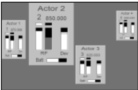
Display of a scene configuration with four actors on the S-MCD Mikroport computer display
